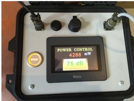
75 dB gain provide 4228 Milli-Watts with -27.5 dBm RF input
