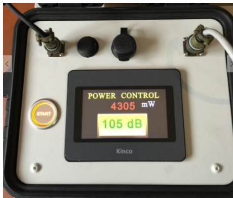
105 dB gain provide 4228 MilliWatts with -69.28 dBm RF input
