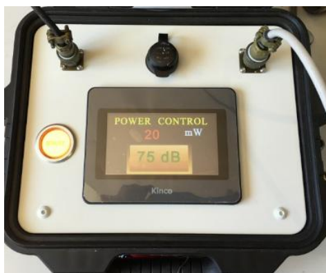
75 dB gain provide 20 milliwatts with -69.28 dBm RF input
